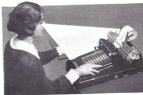
Figure 10—Printing Amounts are visible at three points within easy range of the eyes: on the keyboard, on the roll paper or wide sheet, and in the adding dials where the total is accumulated as amounts are entered in the machine
