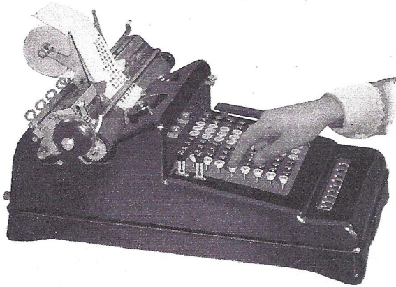
Figure 12—The Flexible Keyboard Little time is lost in correcting mistakes made in depressing keys
